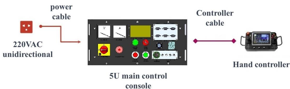
Figure 65 - Manual controller connection diagram.
