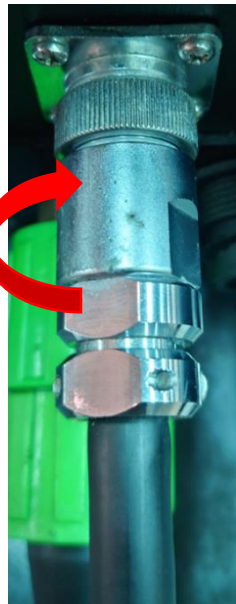
Figure 32 - Rotate clockwise to lock the signal connector in place
