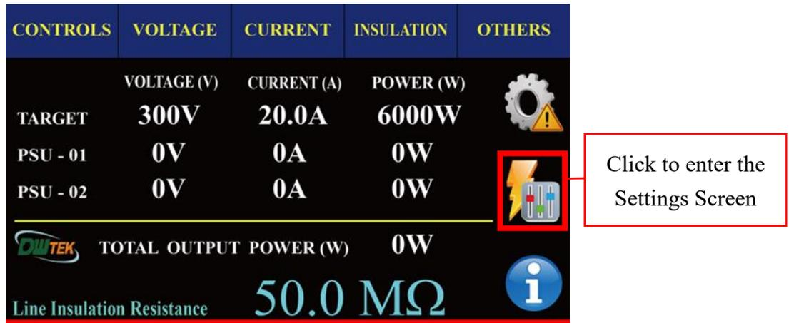
Figure 50 - 5U-Main Console Settings Screen Buttons
