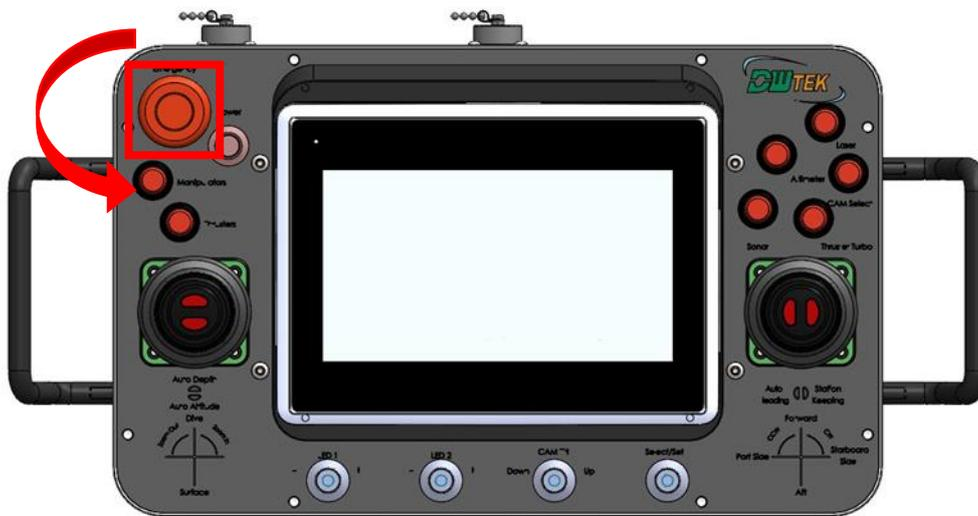
Figure 53 - Diagram of emergency stop switch on manual controller.
