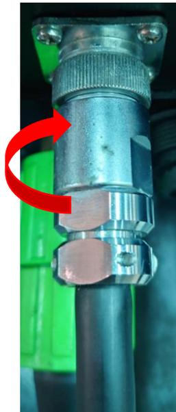
Figure 32 - Rotate clockwise to lock the signal connector in place
