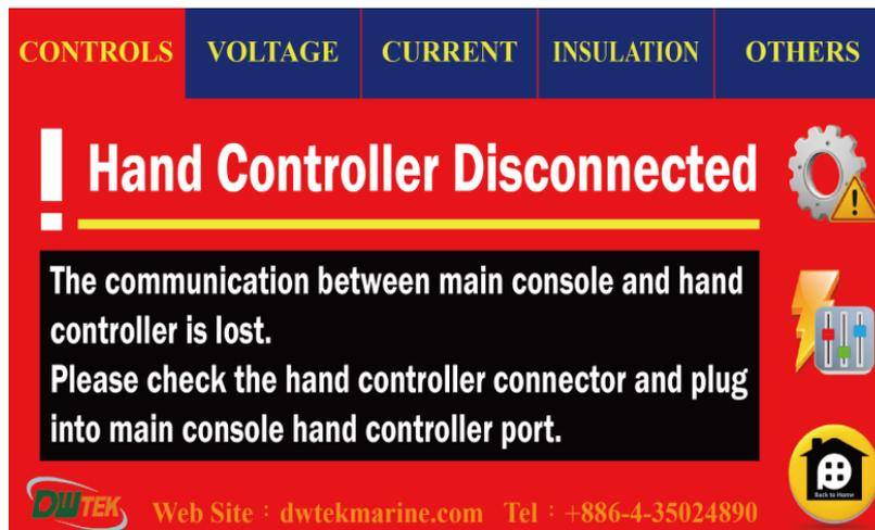
Figure 64 - Manual controller connection abnormal
