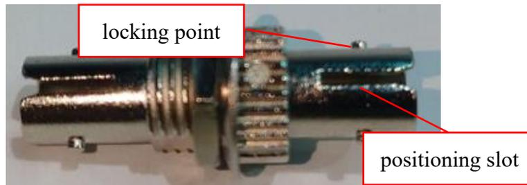
Figure 38 - Fiber signal connector end
