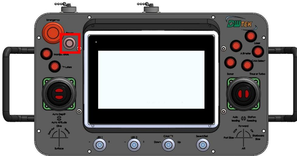
Figure 52 - Hand controller power switch pictorial diagram
