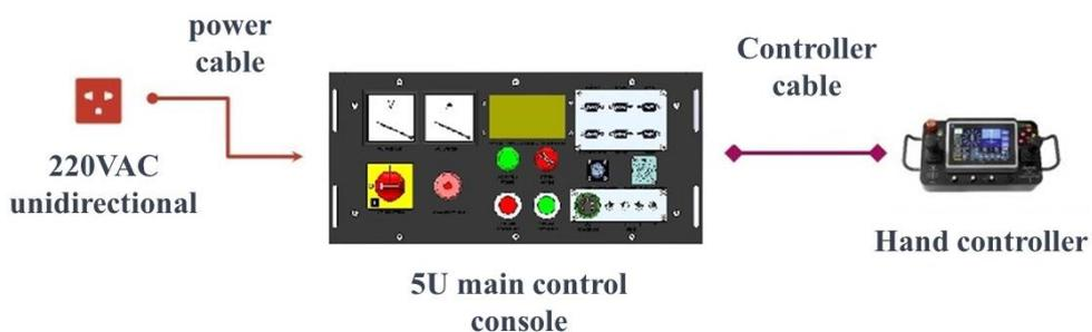
Figure 65 - Manual controller connection diagram.
